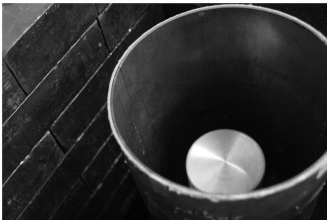
**Fig. 1.** The GEARs detector inside the lead shielding. The Cu/Cd graded-Z shield is visible around the detector can at the center. Contained within the aluminum can is a cryostat which houses the HPGe crystal.
