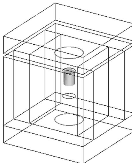
**Fig. 4.** The GEARS geometry implemented in the GEANT4 software package. The box superstructure is lead shielding, the large wire-frame cylinder is the Cu/Cd graded-Z shield, the small wire-frame cylinder is the aluminum can which houses the detector, and the solid cylinder is the HPGe crystal of the GEARS detector.
