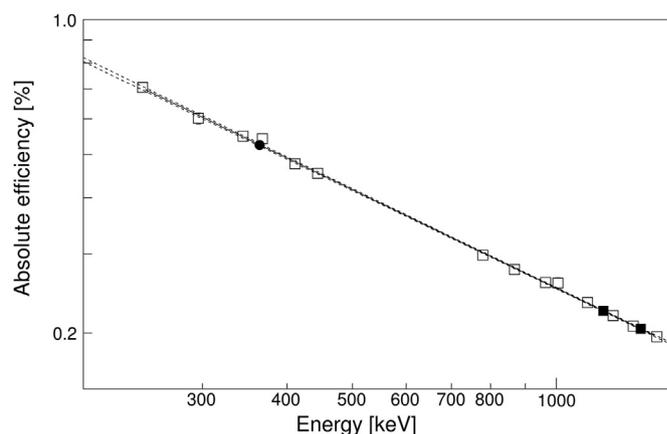
**Fig. 3.** Absolute efficiency of GEARs as a function of energy measured using point sources. The scaled  $\chi^2$  best fit to Eq. (1) is shown as a solid line, the  $1\sigma$  confidence interval is shown as a dashed line. Data shown are  $^{152}\text{Eu}$  [hollow squares], the absolute efficiency measured for  $^{60}\text{Co}$  [filled squares], and calculated absolute efficiency of  $^{131}\text{I}$  peak of interest [filled circle]. The data from this figure are shown in Table 1.
