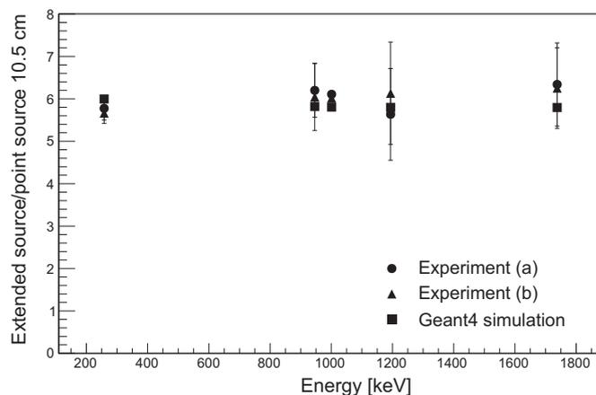
**Fig. 5.** Extended source/point source efficiency ratio at prominent gamma-ray energies of  $^{234}\text{U}$ . The results from two independent experiments (a) and (b) are shown with GEANT4 simulations for the serial dilution measurements described in Sec. 2.3. Results shown are for the 24 mL vial, the initial step of the serial dilution process.
