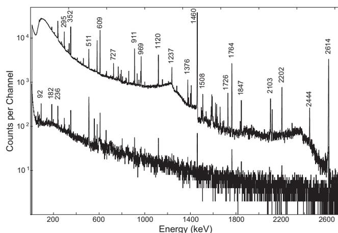
**Fig. 2.** Examples of background spectra obtained with GEARs in an unshielded [top] and shielded [bottom] configuration; the shielded configuration shows a  $\sim 100$  fold decrease in the overall background while many background peaks associated with NORM are either eliminated or strongly suppressed. Spectra are normalized to the same livetime.
